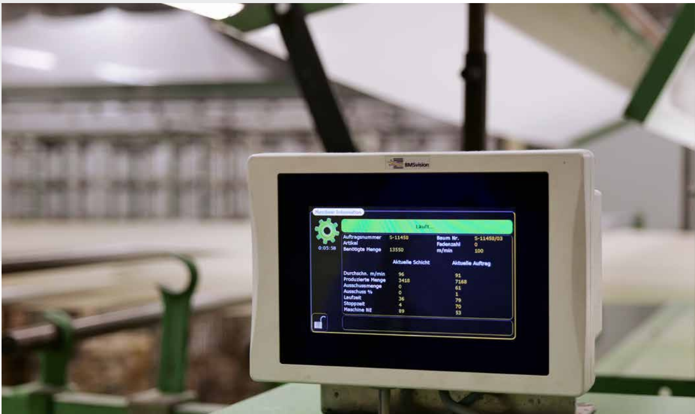
The BMSvision DU11 terminals with 7" touch screen, installed on the warp preparation machines running at Velener transmit machine monitoring data such as speeds and yarn breaks to the WEAVERMASTER Windows server.
