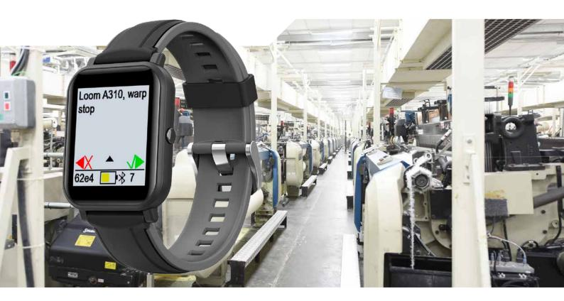
The SMART BRACELET is a wrist wearable device capable of receiving messages from any BMSvision system. Messages are sent based on alarms generated by the BMSvision Events & Alerts module. The device promptly informs operators when there is a need to intervene on a machine.
