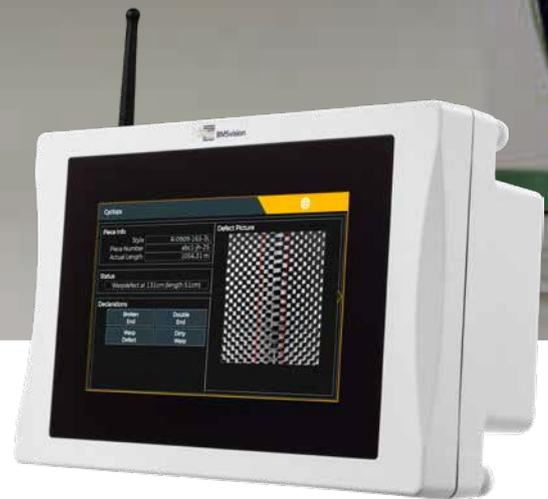
**The Cyclops automatic on-loom fabric inspection system detects warp, filling and point defects by means of a moving camera system installed on the off-loom take up.**
